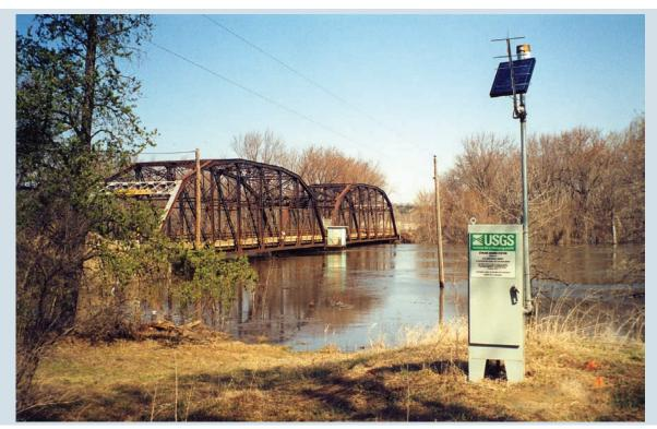
USGS Minnesota stream gage during 2001 spring flood (photograph by Eric S. Wakeman, U.S. Geological Survey).
