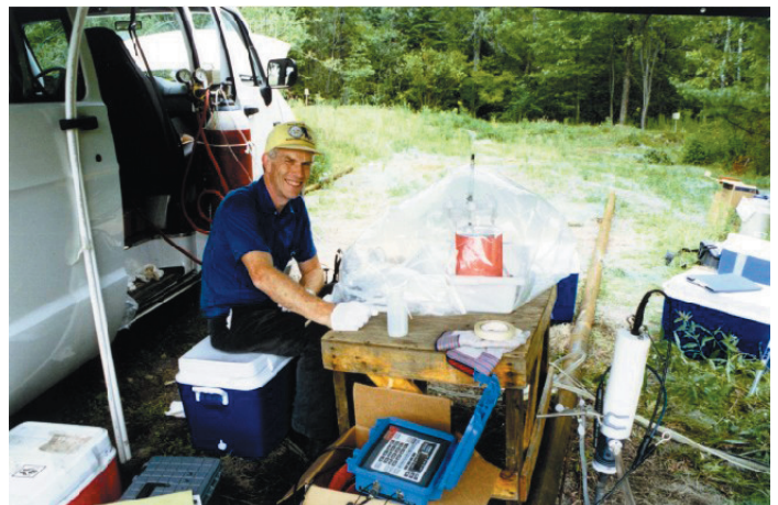
Photo 2. Collection of ground-water samples.
