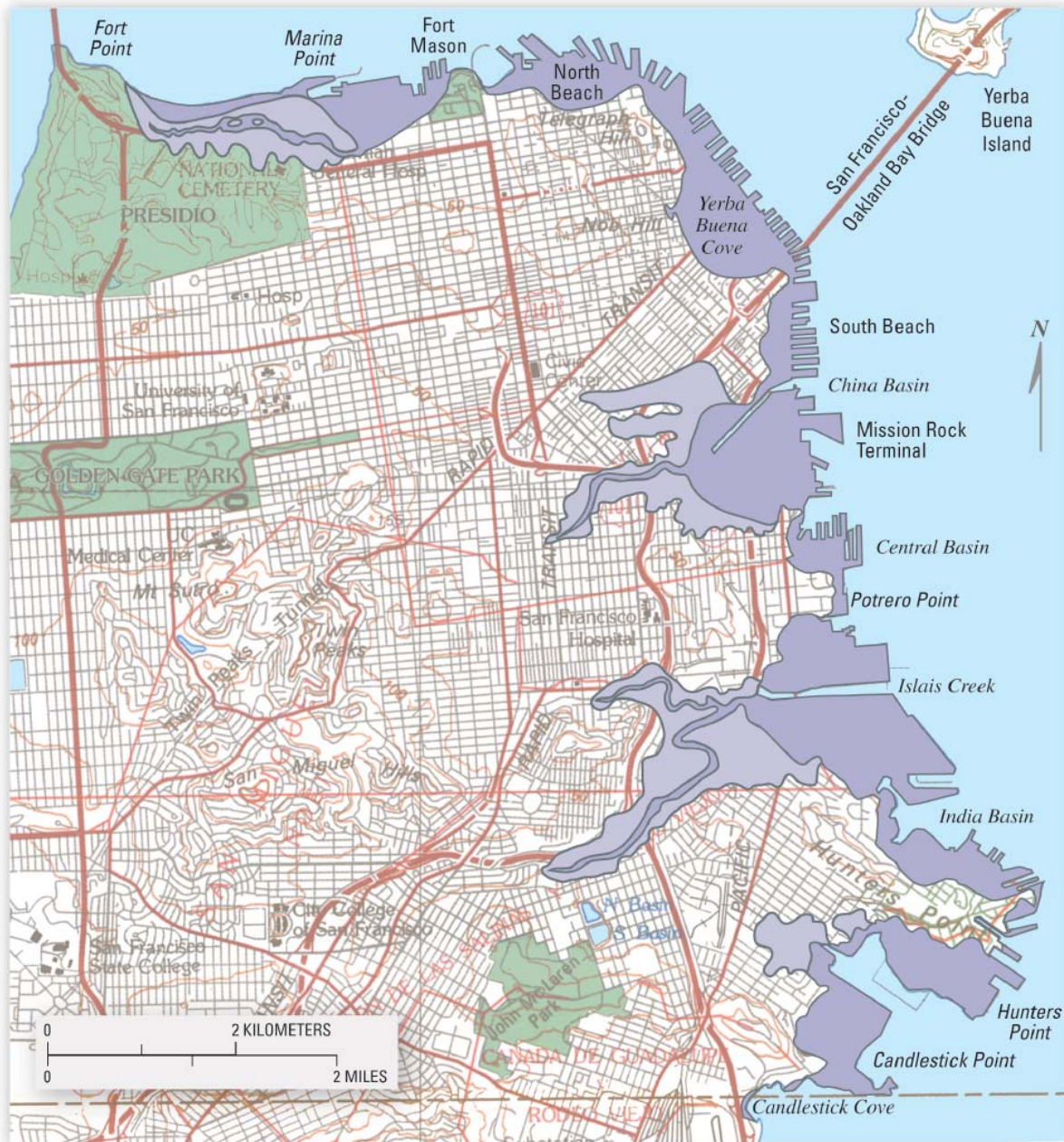
Figure 3. Historical changes to the bay margins in the City of San Francisco. Light purple, tidal marshlands that have been filled since 1847. Dark purple, open water areas filled since 1847. (Modified from Dow, 1973; base map is USGS San Francisco Quadrangle 1:100,000-scale topographic map, 1978 edition.)
