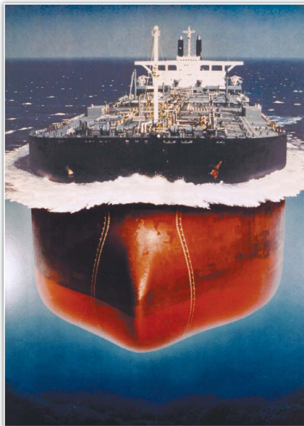
Figure 22. Large, modern oil tankers, when fully loaded, ride low in the water. However, as this combination photograph/diagram shows, the hull of the ship extends several tens of feet below the surface. (Image courtesy of Petroleum Association of Japan.)
